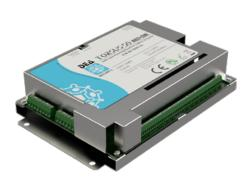
Electronic processing board which manages four TORSUS 50 sensorstrings. It amplifies, digitizes and analyzes the signals coming from the sensor-strings, discriminating the typical signals of an intrusion from those generated by environmental nuisances.
