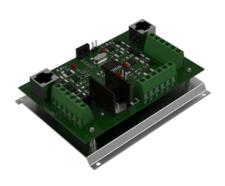
Interconnection board which connects DEA Security processing boards to DEA NET. This board amplifies and regenerates the signals over DEA NET, making it possible to cover long distances.
