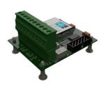
Electronic board which manages a second SERIR 50 sensorstring to protect further 50 metres of perimeter. It must be mounted inside UA-SRC50 Analysis Unit and connected to the processing board.
