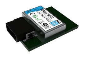
Wi-Fi dongle which connects to the electronic card of SN-SPCP-FDR1, SN-SPCP-FDR1M and SN-SPCP-FWL1 detectors and activates its wireless functionalities. It enables you to configure and calibrate each sensor from tablet or from an Android/IOS smartphone by means of SW-SPCP-APP free mobile app.
