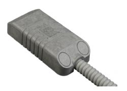
Piezoceramic passive sensor which protects metal burglar bars against shock, cut and breakthrough. Designed for outdoor use, the sensor is protected by a reinforced polyammide housing and the connection cable is wrapped with flexible metal conduit.
