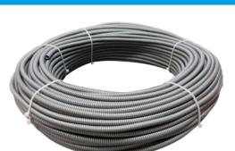
Flexible metal tube for the protection of the connection cable of SN-XS-DR sensors equipped with thicker base. It is made of galvanized steel with single seam, PVC vacuum covered.
