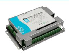
Electronic processing board which manages two SISMA CP 50 sensor-strings. It amplifies, digitizes and analyses the signals coming from the sensors, discriminating the typical signals of an intrusion event from the ones generated by environmental nuisances. The board is equipped with Ethernet interface and IP native support.
