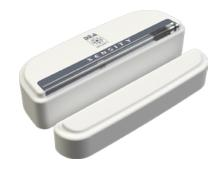
Dual-tech microprocessor detector for the Point ID protection of windows and doors against burglary, opening, breaking through and drilling. It can be installed in any inclination and orientation and it is available with either thicker or thinner fixing base: the thicker base is compatible with the connection cable wrapped with flexible metal conduit.
