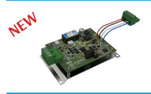
Electronic board which galvanically isolates the CU-FSP2P control unit from the sensor-strings connected to a bus. It prevents possible electric problems (interferences, overvoltages, shortcircuits or earth issues) from propagating from the control board to the sensor bus and viceversa.
