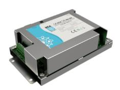
Electronic processing board which manages two SERIR 50 sensor-strings.
