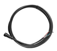
5-metre connectorized cable for the connection of the CU-FSP2P control unit or the BR-FSP2PLT-CTRL control board to the first connectorized sensor-string of a bus (LN-FSP2P/LN-FSP2P-A strings or SN-FSP2P/SN-FSP2P-A sensors equipped with CN-FSP2P connectors).
