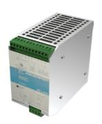
Stabilized switching power supply unit (mark Adelsystem) with 24 Vdc output voltage and 3 A max output current. It provides two relay outputs: one for mains or backup and one for low or discharged battery.
