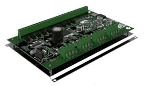
Multi-zone digital processing board to manage all SERIE A03 PRO sensor models. It processes the signals coming from the detectors and generates alarm states. The service app displays the alarms differentiating them by type of attack: shock (low shocks), breakthrough (gross attacks), drilling (continuous shocks).
