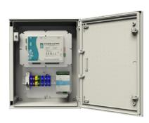
The control unit manages up to 300 detectors on 2 communication buses for maximum 1.500 metres of perimeter if the spacing between the sensors is 5 metres and 900 metres of perimeter if the spacing is 3 metres. Besides enabling the configuration of the detectors by means of a service software, the control unit automatically recognizes and sorts the field detectors and raises the alarm signals.
