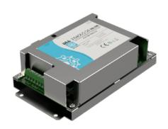
Electronic processing board which manages two TORSUS 50 sensorstrings. It amplifies, digitizes and analyzes the signals coming from the sensor-strings, discriminating the typical signals of an intrusion from those generated by environmental nuisances. The board is equipped with Ethernet interface and IP Native support.
