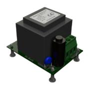
Current transformer inside the Analysis Unit.
