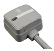
Microprocessor analysis board for SN-XS-GR sensors. It processes the analog signals coming from SN-XS-GR sensor and sends the alarm signals (if any) to the Controller board through XENSITY Bus. BR-XS-GR can discriminate between cut (continuous vibrations), shock (weak impacts) and breakthrough (strong impacts); it also allows filtering nuisance alarms due to thermal expansion of the metal structure.
