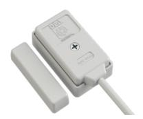
Piezodynamic shock detector to protect windows and doors against shocks, opening and breakthrough attempts. Door, window or skylight frame mounted, its high detection capability enables it to protect the whole structure, including glasses.
