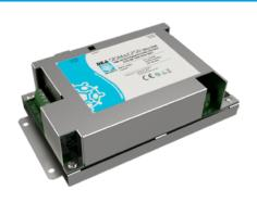
Electronic processing board which manages one SISMA CP 50 sensorstring. It amplifies, digitizes and analyzes the signals coming from the sensors, discriminating the typical signals of an intrusion from those generated by environmental nuisances. The board is equipped with Ethernet interface and IP Native support.
