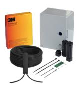
Module for the protection of a rigid fence up to 50 metres long. It is composed of a prewired sensor-string of 20 sensors for the protection of fence panels with 2.5 metres width, a preassembled Analysis Unit, a 25-metre hank of cable and a wiring kit.
