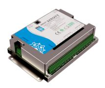
Controller board which manages up to 32 XENSITY sensors/peripheral devices, among which a maximum of 24 BR-XS-SMCAPU boards. It has the function to supply power, check the operating status and receive signals from each device connected to the bus, store them in an internal memory making this information available through relay contacts, DEA NET proprietary network or IP network.
