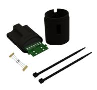
Peripheral module containing an electronic interface board for the management of a resistive balanced input. It can be connected everywhere along the sensor-string and allows you to integrate into the system signals coming from third-party devices such as magnetic contacts. The printed circuit board is protected by a polyamide housing which provides a very high resistance to UV rays and scratch.
